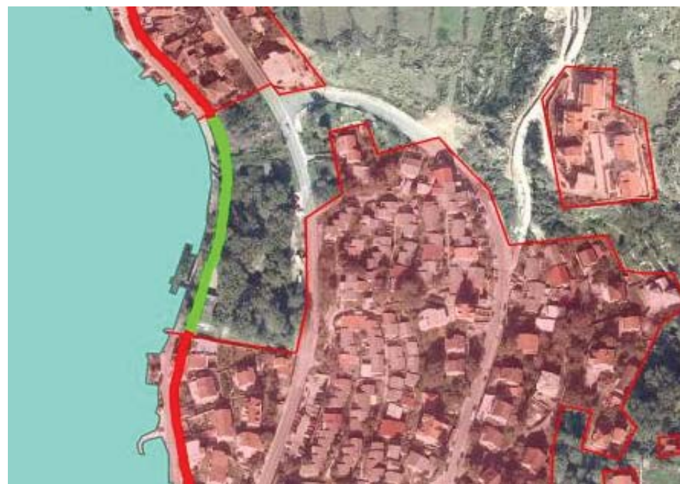
Figure 6.1: Method of calculating the length of land built along the coast: the overlap of the constructed parts of the construction area (red polygons in the orthophoto) and the generalized shoreline gives the length of the constructed shore (red line)
