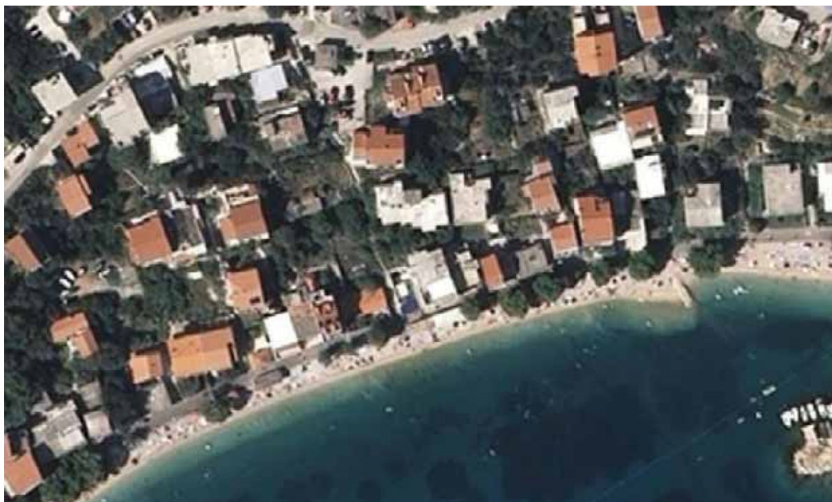
Illustration 1: Example of a situation of newer construction with minimum setback (cca 15 m) which reduced surface and capacity of the beach and of the narrow coastal belt to a minimum (Igrane, Podgora Municipality, Splitsko-dalmatinska County, source: http://geoportal.dgu.hr ).
