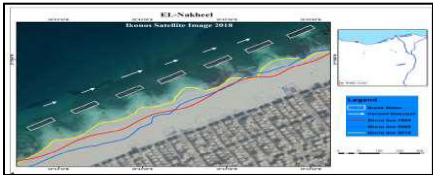
Fig (5): The shoreline changes at El-Nakheel beach from 1984 to 2018. Source: Salama et al (2021).
