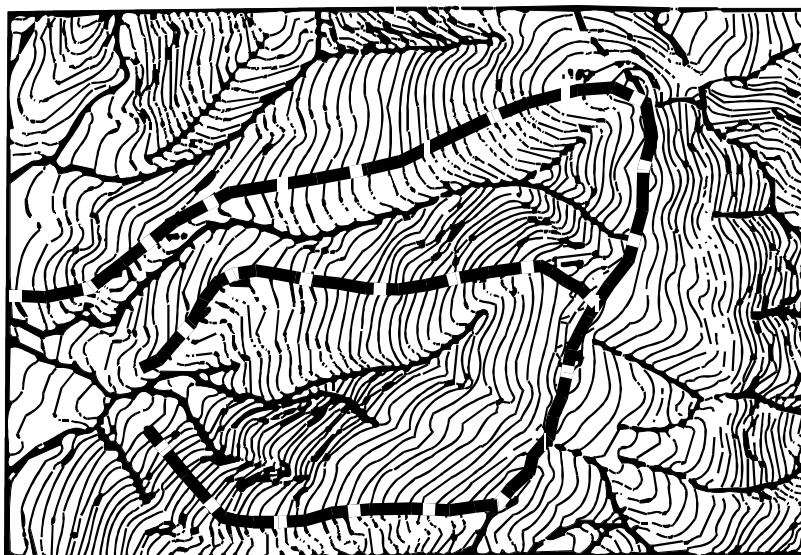
Figure I-3. Identification of divide lines
