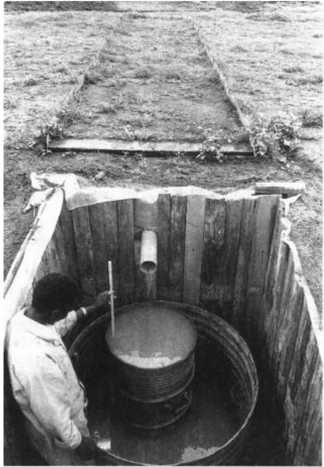
Figure II-1. Total collection tanks
