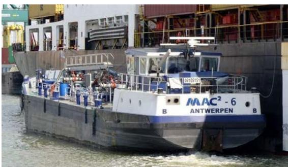
Barge collecting liquid oily waste
