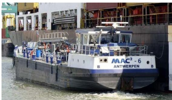
Barge collecting liquid oily waste
