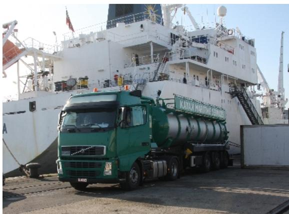
Tank truck collecting oily waste
