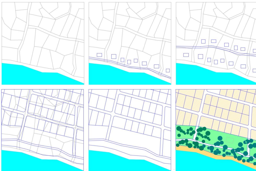
Figure 8. Schematic representation of the land redistribution that allows designing a coastal setback regime (Adapted from JICA)
