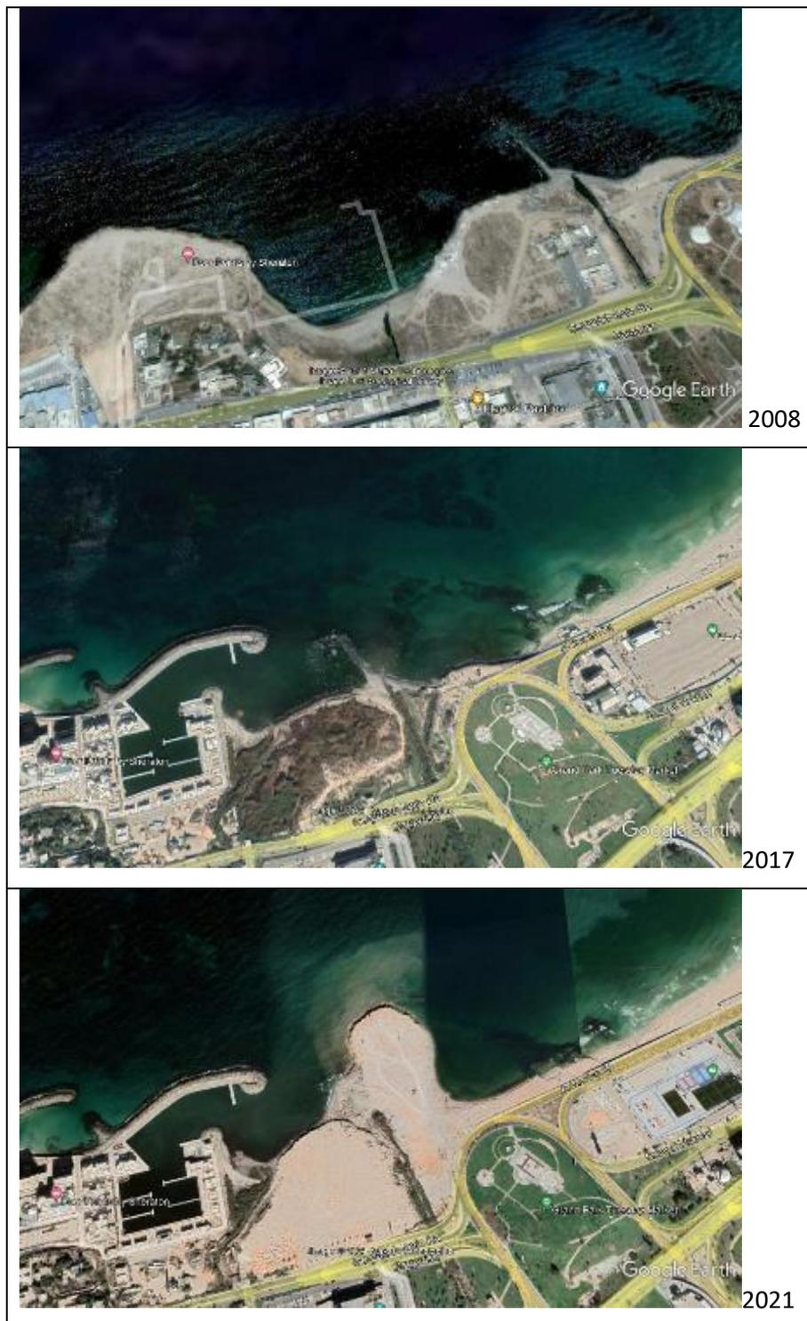
Figure 9 Construction of Tripoli Marina, note the site in 2008 as a natural small bay, then between 2009- 2017 works completed, later in 2021, to the east of the marina dumping of coastal waters using building demolition materials, note the turbidity caused.
