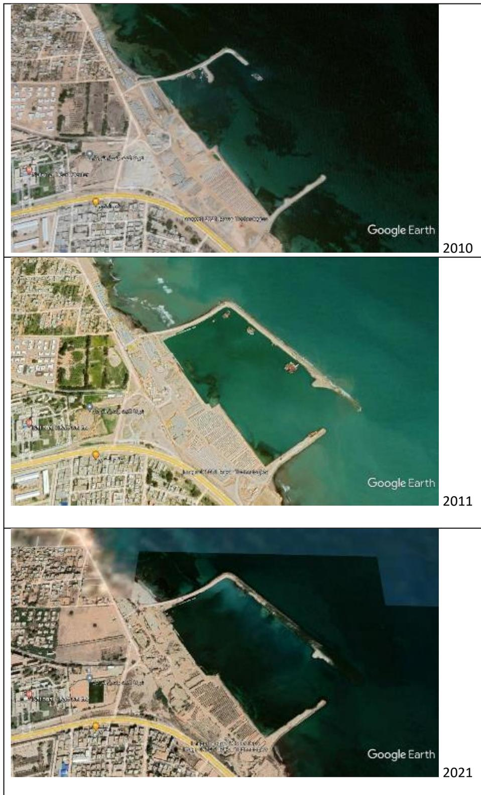
Figure 10 Commercial port of Tajura from construction of breakwaters in 2010 then mostly ready in 2011, but later due to departure of construction company in 2011 the project was not completed, and the construction is breaking down in 2021.
