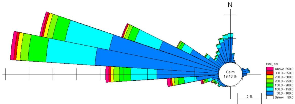
**Figure 13.** Annual rose diagram of significant wave height (cm) in deep water offshore Haifa, recorded by CAMERI in the period of 1.11.1993 - 31.3.2015
