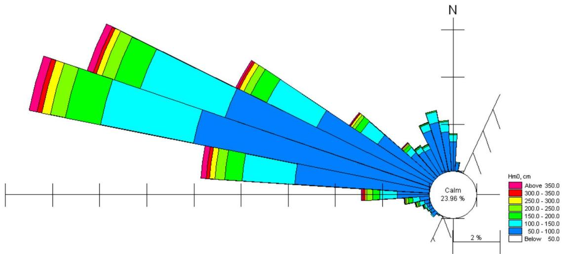
**Figure 12.** Annual rose diagram of significant wave height (cm) in deep water offshore Ashdod, recorded by CAMERI in the period of 1.4.1992 - 31.3.2015 (Levin et al., 2012a)
