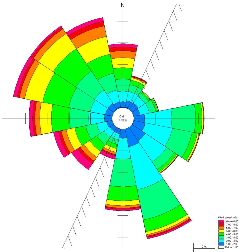
**Figure 8.** Wind rose diagram for 18 years (1.4.1993-31.3.2011) of 10 min averaged wind records at Ashdod (Levin et al., 2012a)
