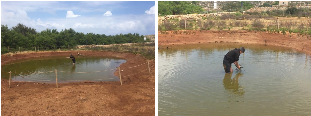
Figure 6: Use of probes was employed to test water quality in the artificial pool on two specific occasions, that is, during a prolonged dry period (May 6 th ) and immediately after a rain episode (May 10 th ).
